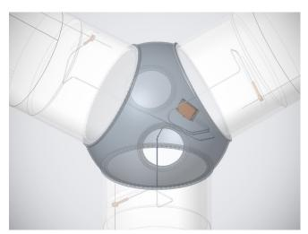
The Lightning Key Data System is integrated in the wind turbine hub and blade area and is designed to withstand harsh environments. One sensor in each blade gives momentary measurements of the lightning behavior during a strike.
